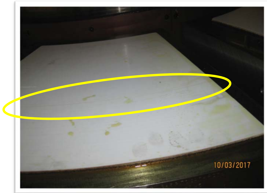
Photo 16: Heavy grooving on PTFE surface
