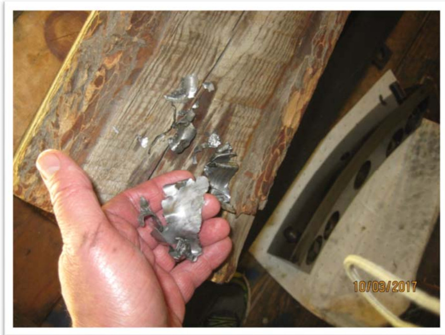
Photo 14: Babbitt removed from the bearing pot
