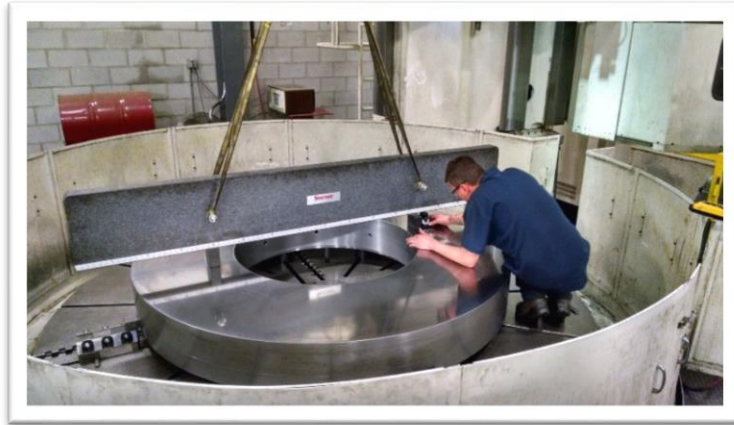
Photo 1 - Measuring the Runner Plate Flatness
