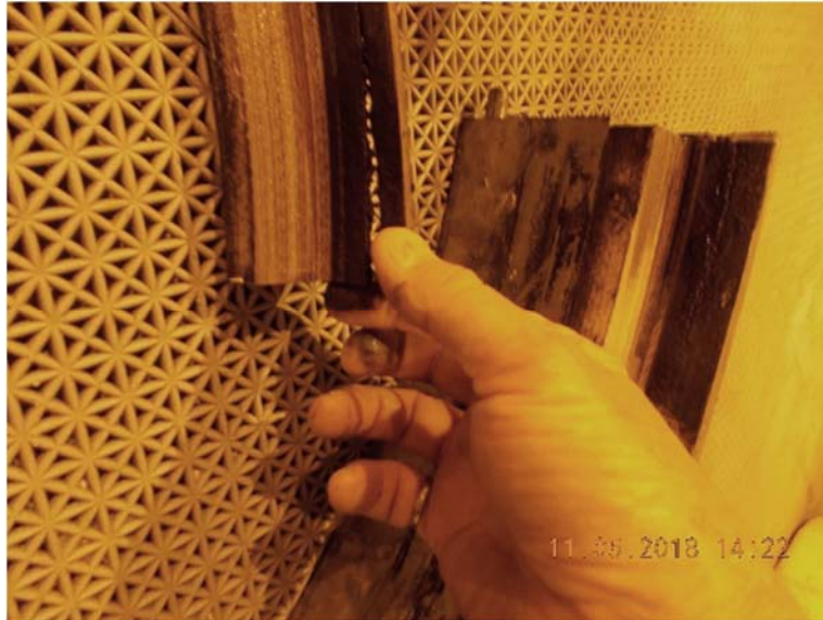
Photo 18: Worn L/D seal element after removal from piston
