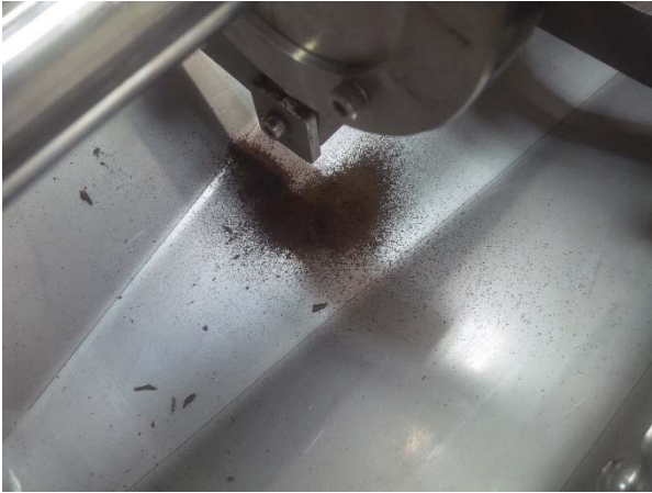
Photo 24: Worn LD material ring #4
