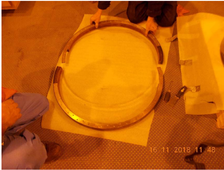
Photo 20: Segmented Lignum Vitae seal element with bronze backing rings
