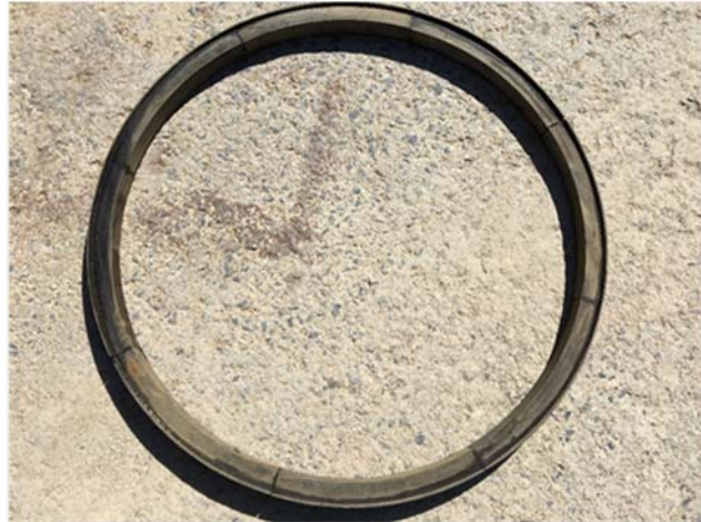
Photo 27: Lignum Vitae seal after 1400 hours operating time
