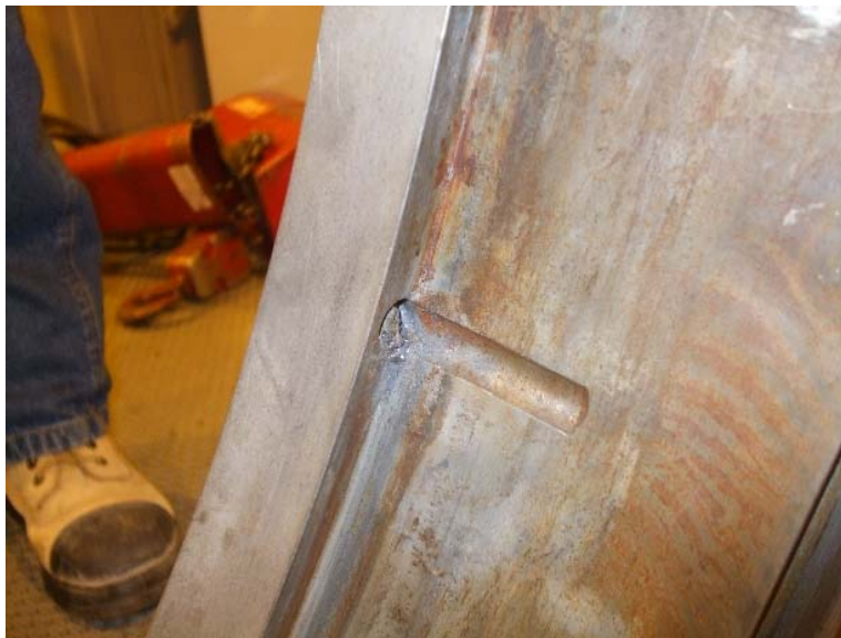
Photos 13: Blocked pressure monitoring port
