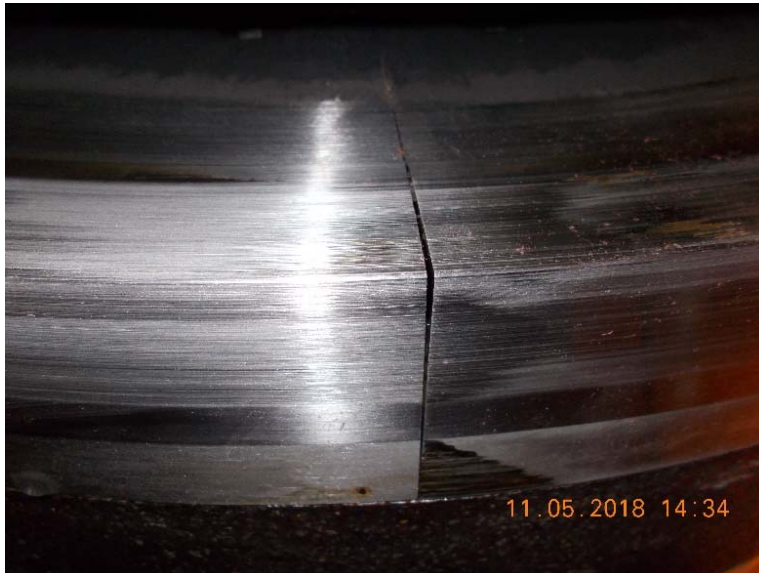
Photo 5 – Gap and sharp edges act as a scraper on the seal element
