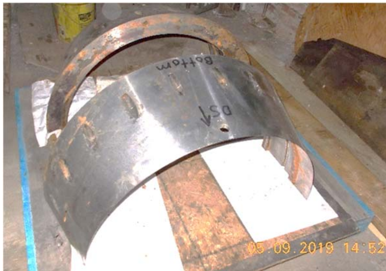
Photo 26: Outer seal cover with no evidence of twisting or pick up
