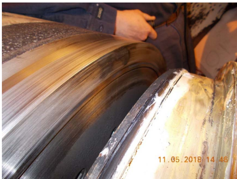
Photo 6: Burn marks on thrust flange.
