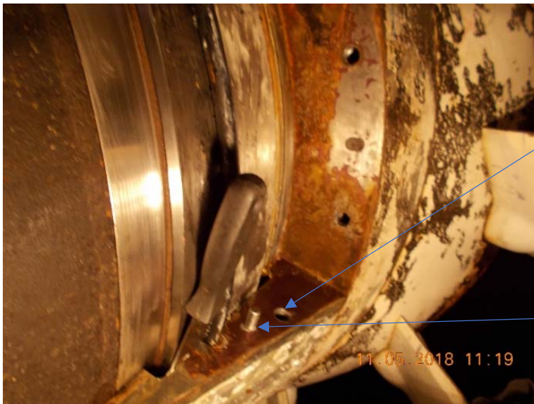
Photo 4: Lower half of outer seal cover
