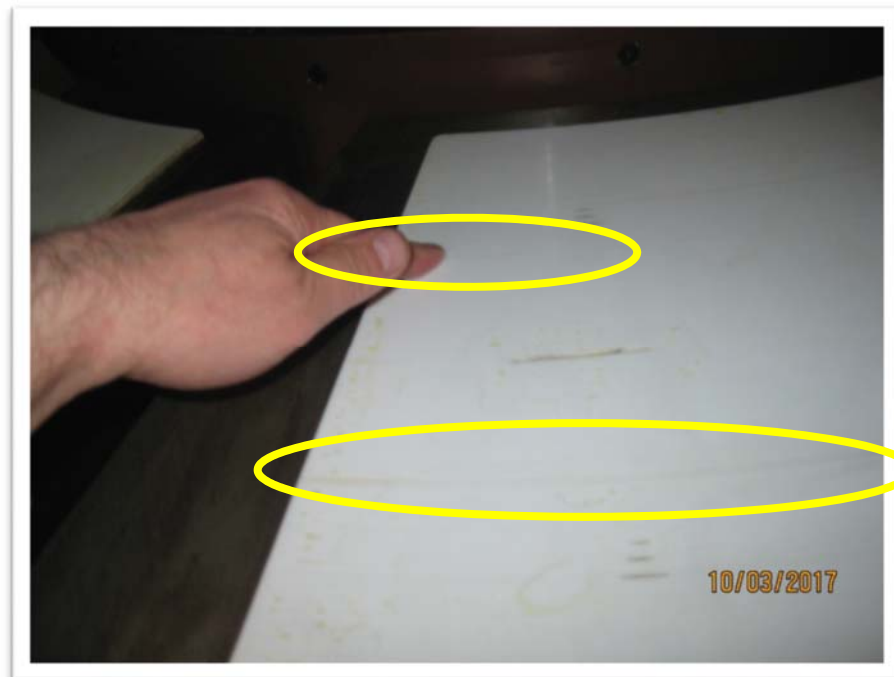
Photo 15: Heavy grooving on the PTFE surface. One wear mark removed. Only 0.002 inches of material was worn.
