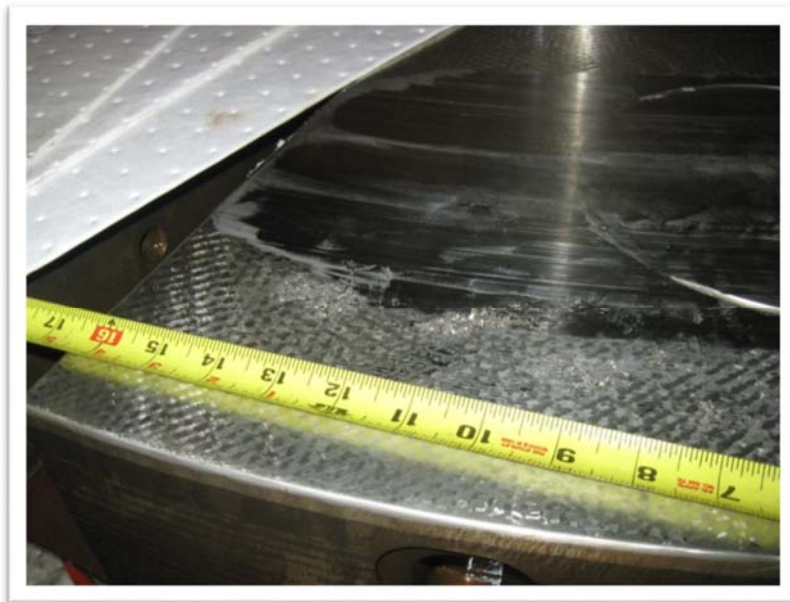
Photo 5: Wiped thrust bearing
