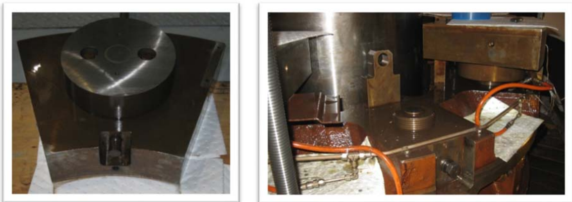
Photos 10 & 11: Bearing support directly in the center of bearing pad
