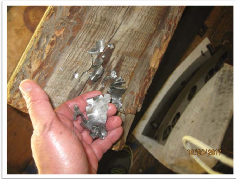
Photo 14: Babbitt removed from the bearing pot
