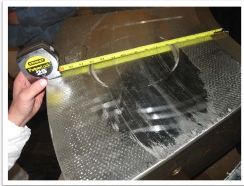
Photo 4: Wiped thrust bearing
