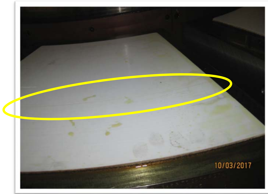
Photo 16: Heavy grooving on PTFE surface
