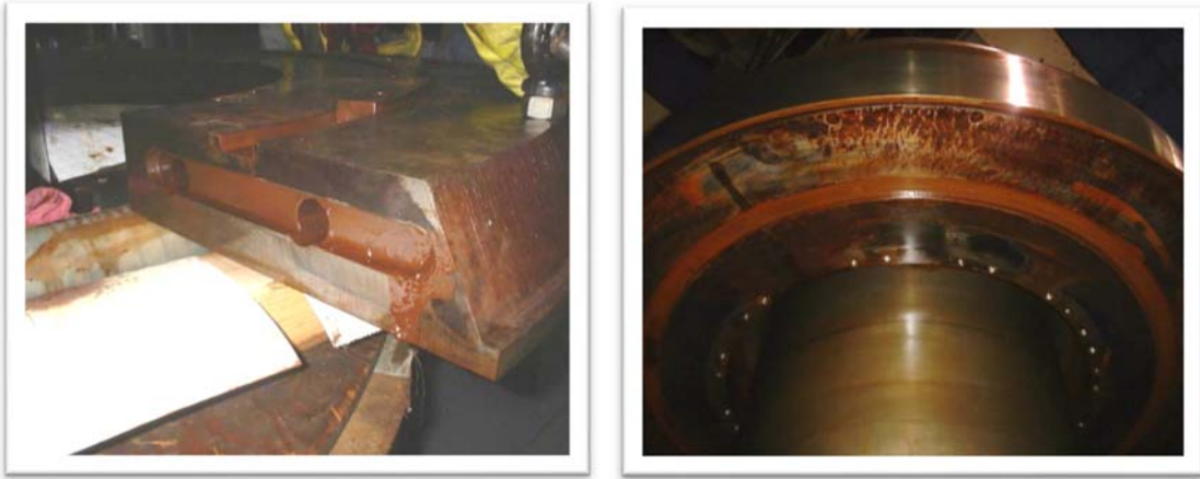
Photos 1 & 2: Fretting at the runner plate split key and the thrust block mounting face 2006
