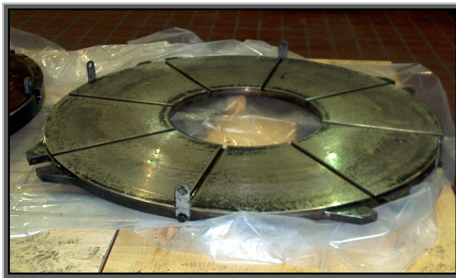
Figure 4. Babbitted Bearing Plate - Flat, Spring Supported Style
