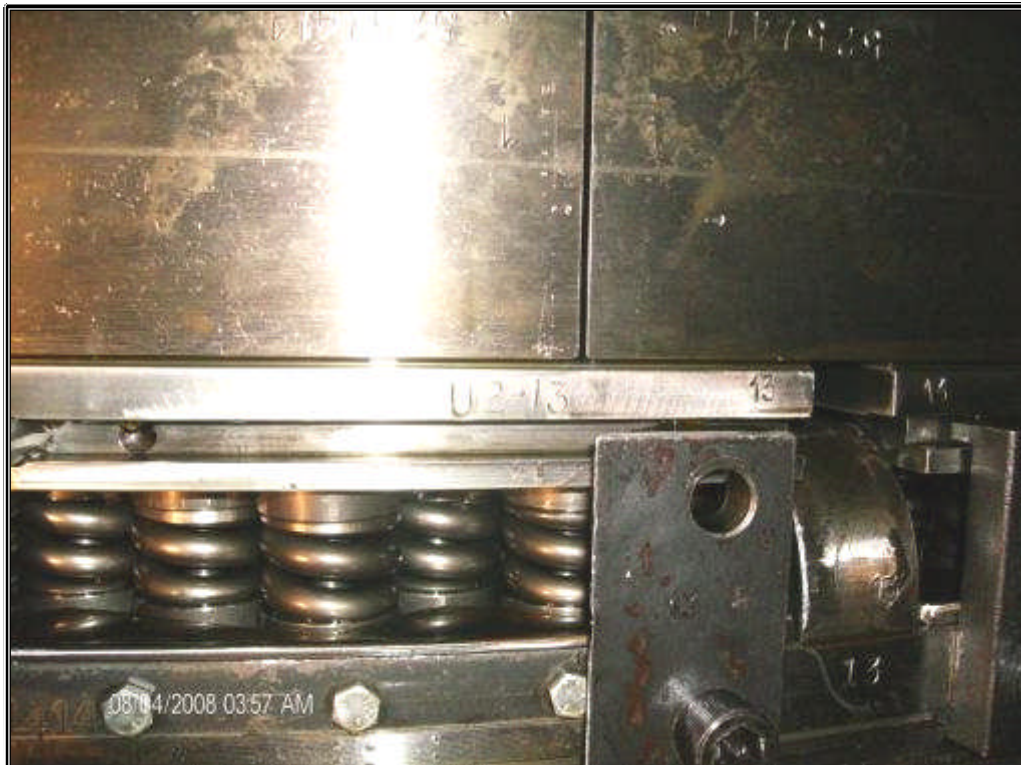
Photo 2 Old Runner Plate With Gap Between Segments
